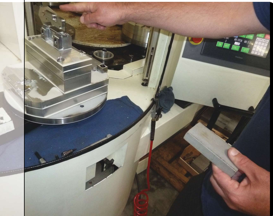
A blank is loaded onto a pallet with three different fixtures (the second fixture is raised at center, with the first and third on either side), allowing the part to be completely machined on the same pallet.
